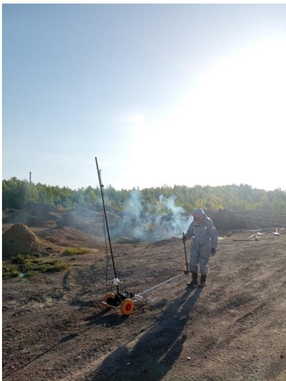
Figure 4. Conducting measurements with a magnetometer on heaps using a diamagnetic frame. The measurements in the photo are carried out by Natalia Godlewska.
